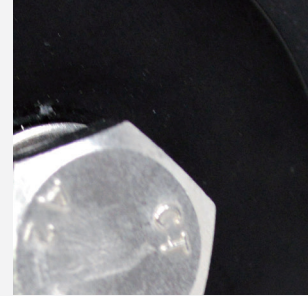
Use 304 stainless steel screws
